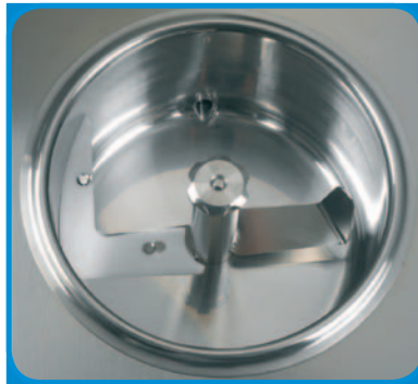
• Cylinder and beater detailed view
